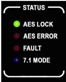
**AES LOCK** - Green LED indicator illuminates when UpMix has acquired a valid AES3 digital input signal.
